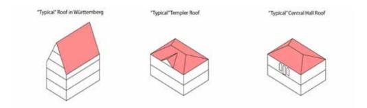
Figure 5. Roof types showing the connection between the Templer house origin and the local central hall typology. Illustration by author.
