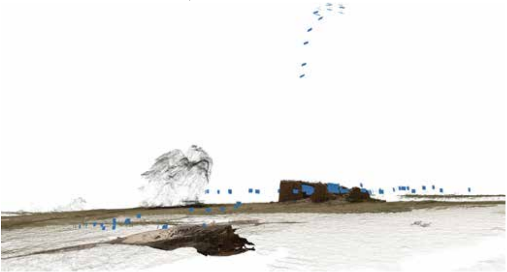
Figure 5. The Bayka (stone house) and storage cave of Ibn Bari, al-‘Araqib: point-cloud composite with camera locations. Photo by author, Forensic Architecture, 2017.
